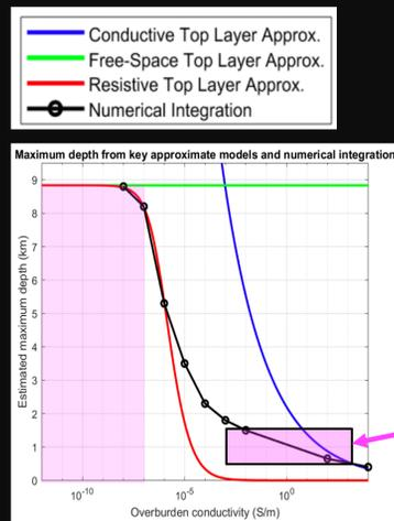
Conditions on Mars (low surface temperature, low EM noise levels, dry overburden crust) allow TEM sounding to a depth ~10x deeper on Mars than on Earth with similar mass/power resources.
